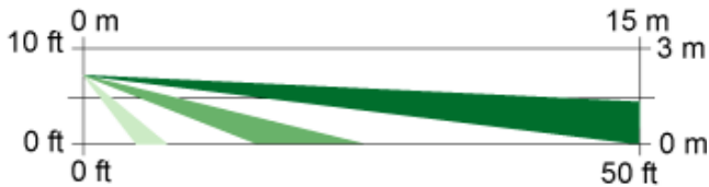
Side View Standard Broad Coverage: 9 m to 15 m x 15 m (30 ft to 50 ft x 50 ft)
